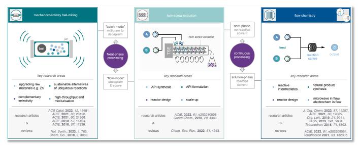
The potential solvent savings afforded by mechanochemistry techniques are particularly appealing at larger scales, yet the absence of a bulk solvent to dissipate heat makes a batch milling process particularly hazardous. This talk will focus on developments in continuous mechanochemistry through the technique of reactive extrusion.
